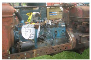
The first thing I noticed about this straight eight was the 1954-only spark plug wire loom, which may indicate the model year of this engine. The second thing I noticed was the lack of the factory starter, a custom made plate has been installed on the back of the block. See below, the original starter mounted on top of the bell housing under the fuel tank. Pete
