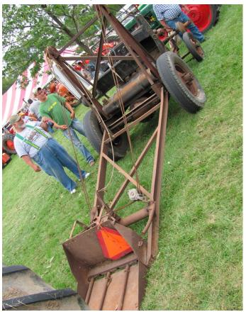
The first was a 1929 Pontiac, which had been stripped down years ago and configured with a long boom out the rear. This was raised and lowered by a cable system, driven off of a second differential mounted in front of the radiator!! Its ignominious fate in life was to scoop manure. I'll leave it to someone with more manure experience to try to explain the mechanism.
