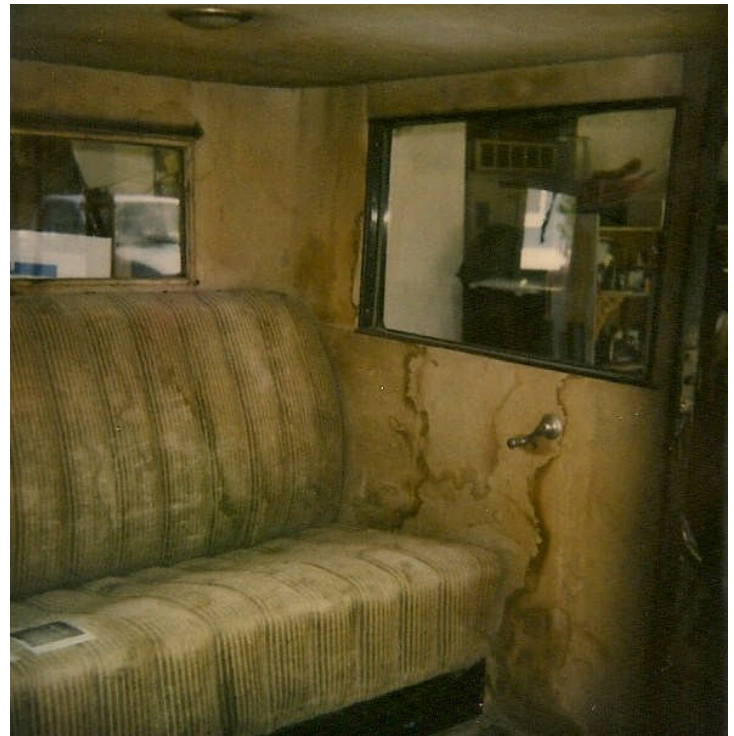
The rear passenger compartment showing obvious signs of water damage, but otherwise surprisingly intact for a 1926 automobile.
